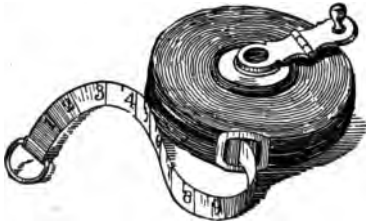
FIG. 48. A tape-measure. Short tapes a yard (3 feet; 36 inches) long are used by salesmen to measure cloth or ribbons. Longer tapes (50 or 100 feet long) are used by carpenters and masons. Tapes made of flexible steel are used by surveyors to measure land, lay out streets and so forth.
